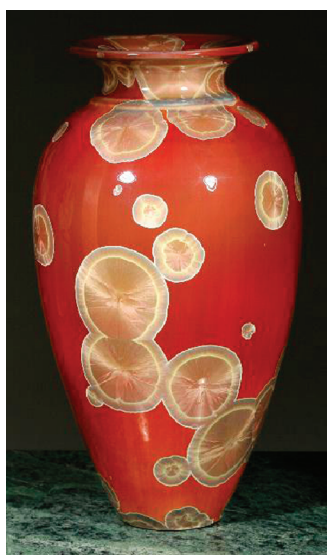
Figure 33. Willemite ( \alpha - \text{Zn}_2\text{SiO}_4 ) spherulites in crystalline glaze. Ceramic by John Mankameyer. Photo reproduced with permission of John Mankameyer, Miles City, Montana.
